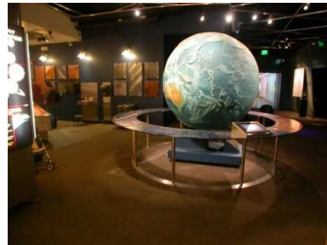
Figure 4 - Information Ring Not Cane Detectable
